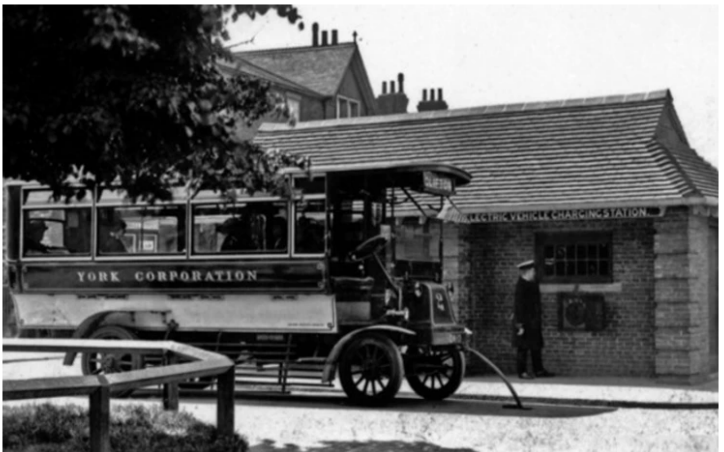
York battery bus recharging at Clifton Green "Electric Vehicle Charging Station" in 1915. These operated from 1915 to about 1920.
